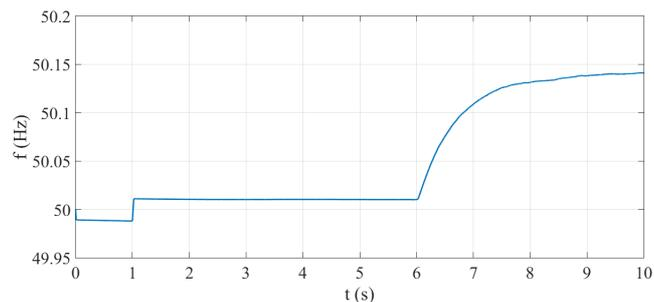
Fig. 12. The region frequency curve during FCP of the PV power plant.
