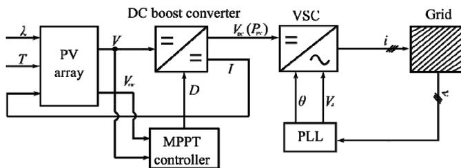
Fig. 2. The block diagram of the PV power plant model.
