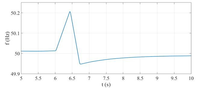
Fig. 7. Frequency's changes due to PV power plant disconnection
