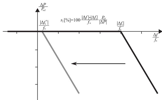
Fig. 10. Active power frequency response capability of power generating modules in overfrequency mode with the lower threshold limit.
