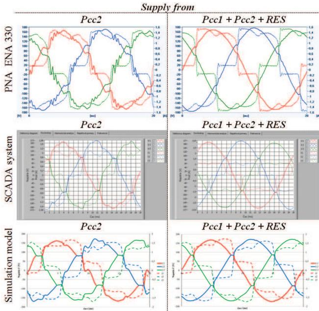
Fig. 8. Waveforms comparison among different systems
