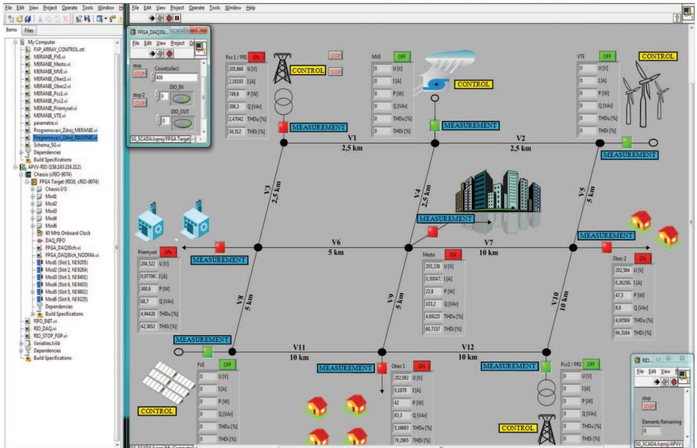
Fig. 1. Developed SCADA system
