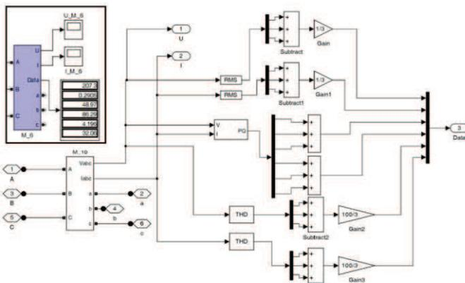
Fig. 6. Measurement unit in the simulation model
