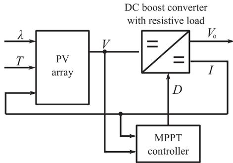
Fig. 9. A block diagram of PV system.
