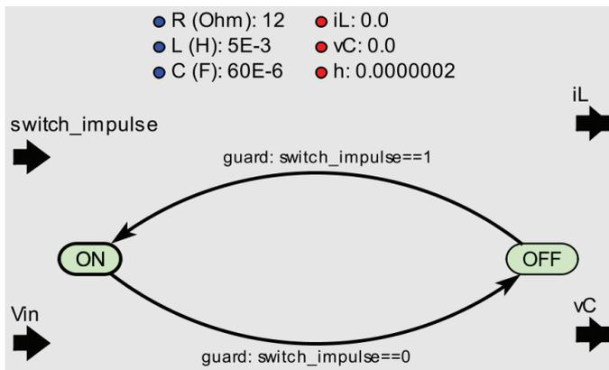
Fig. 6. FSM model of a DC boost converter.
