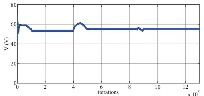
Fig. 12. PV array output voltage feeding the converter for different solar irradiances.
