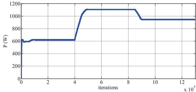
Fig. 14. PV array output power for different solar irradiances.
