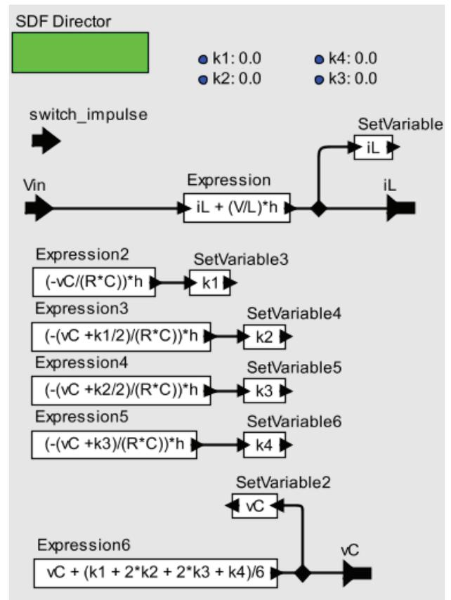
Fig. 7. ON state of the converter.
