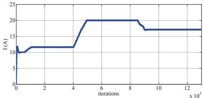
Fig. 15. PV array output current for different solar irradiances.
