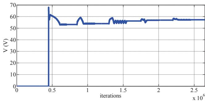
Fig. 18. PV array output voltage calculated by FSM model of PV system.
