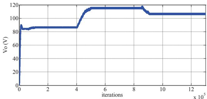
Fig. 16. DC boost converter output voltage for different solar irradiances.
