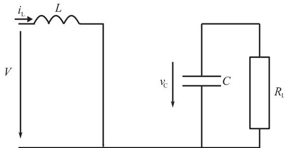
Fig. 3. ON operation mode of a converter.
