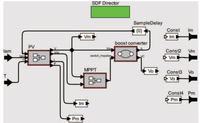
Fig. 11. Model of PV system.
