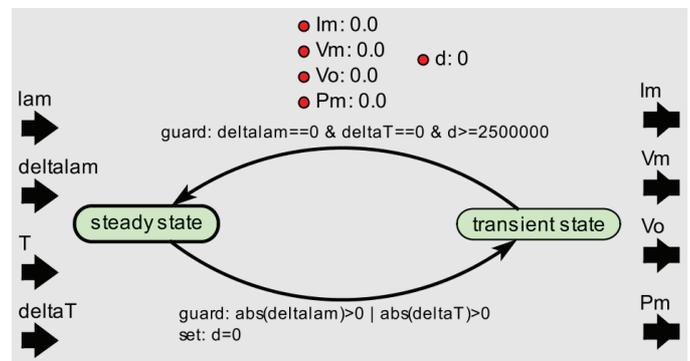
Fig. 17. FSM model of PV system.
