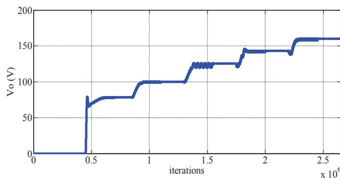
Fig. 21. DC boost converter output voltage calculated by FSM model of PV system.
