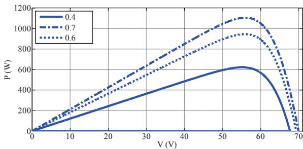
Fig. 10. P-V curve of the PV array.
