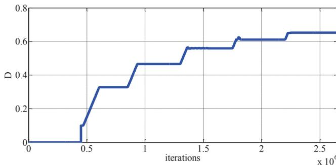
Fig. 19. Changes of duty cycle in FSM model of PV system.
