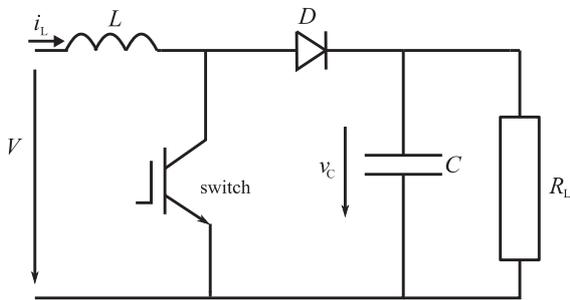
Fig. 2. Topology of a DC boost converter.
