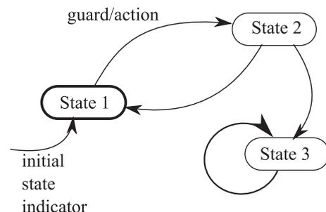
Fig. 1. A graphical notation for FSM.
