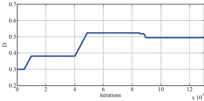
Fig. 13. Changes of duty cycle of the converter for different solar irradiances.
