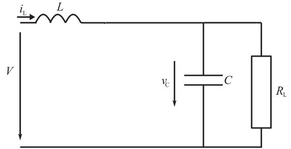
Fig. 4. OFF operation mode of a converter.
