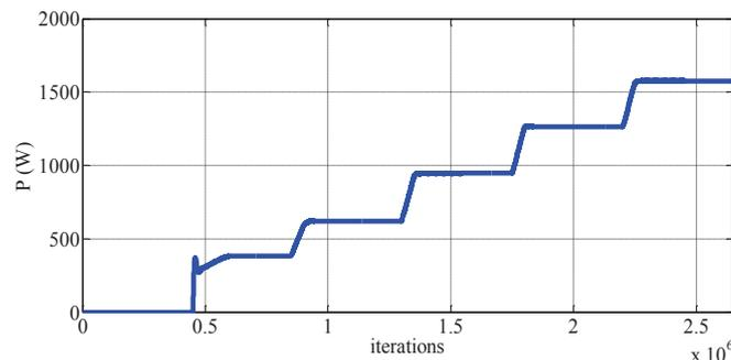
Fig. 20. PV system's power curve calculated by FSM model of PV system.
