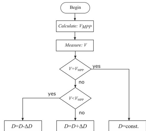
Fig. 5. Flowchart of the constant voltage method.
