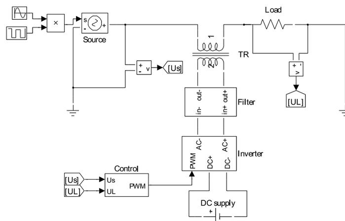
Fig. 3. Simulation model of DVR in Simulink
