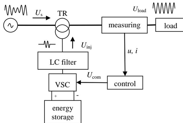
**Fig. 1.** Simplified scheme of a DVR
