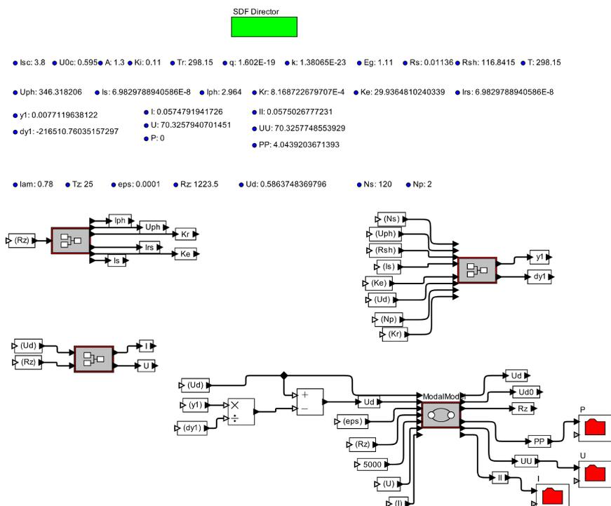
Fig. 3. Model of a PV panel created in Ptolemy II
