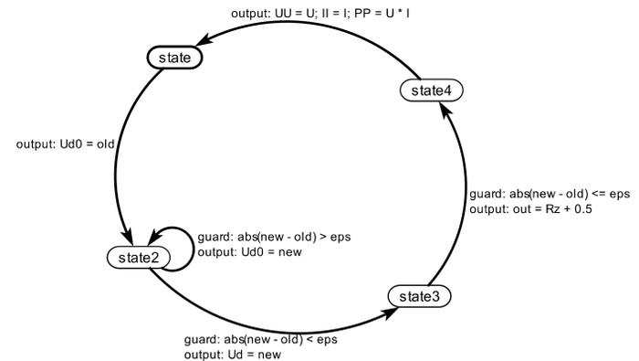
Fig. 4. FSM diagram in the model of PV panel
