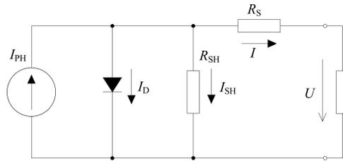
Fig. 1. Equivalent model of a photovoltaic cell with resistive load
